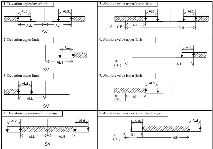
: Temperature alarm output operation range ALL: Alarm output lower limit setting ALH: Alarm output upper limit setting ALd: Alarm output sensitivity
