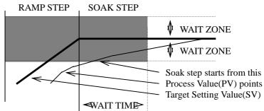
: Wait time... This means the maximum waiting period to start next step when PV(Process Value) does not reach to the SV(Setting Value).
