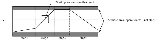
$\underline{SV\;start}\;\dots$  .At the set time of Step 1, operation starts from the specified SV(Set Value) to the target set value(SV1) of Step 1.
