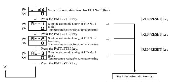
When the automatic tuning is complete, the product will switch back to the automatic tuning startup screen.
