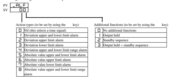
Alarm temperature setting mode (The SET lamp lights.)
