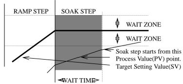
• SV start • • It will start from the setting value at the starting time of operation which to be treated as the PV(Process Value) or the target SV(Setting Value).
